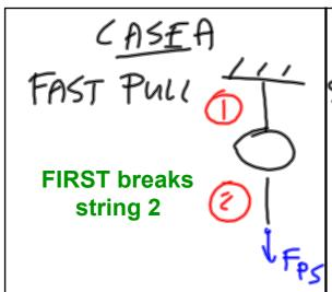
Inertia of the ball (measured by its mass; ability to resist the acceleration) prevents the transfer of F<sub>PS</sub> from string 2 to string 1.
