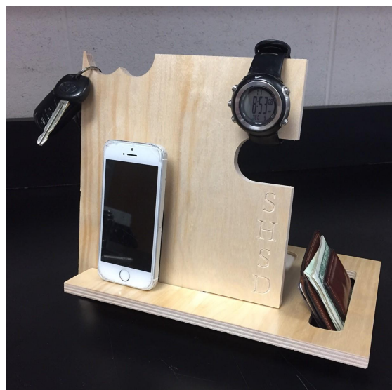
Catchall cut on CNC Router
